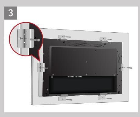
Fasten the screw to fix the bracket to the panel
